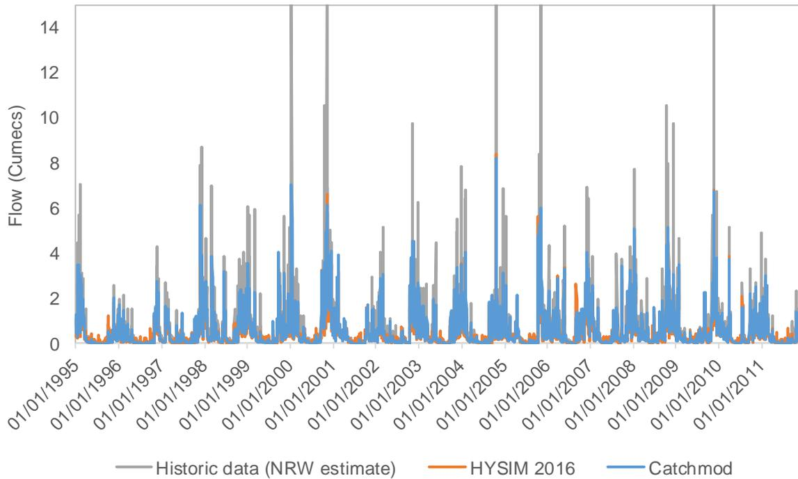
Figure 6.8 - Observed and simulated (HYSIM 2016 and Catchmod) flows for Llyn Alaw
