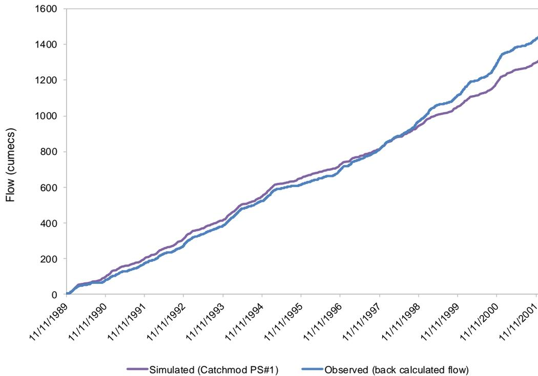
Figure 4.16 - Volumetric fit for Cwmystradllyn reservoir catchment
