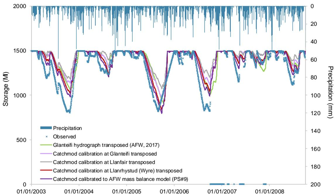
Figure B.10 - Observed and modelled storages for Teifi Pools for 01/2004-09/2008
