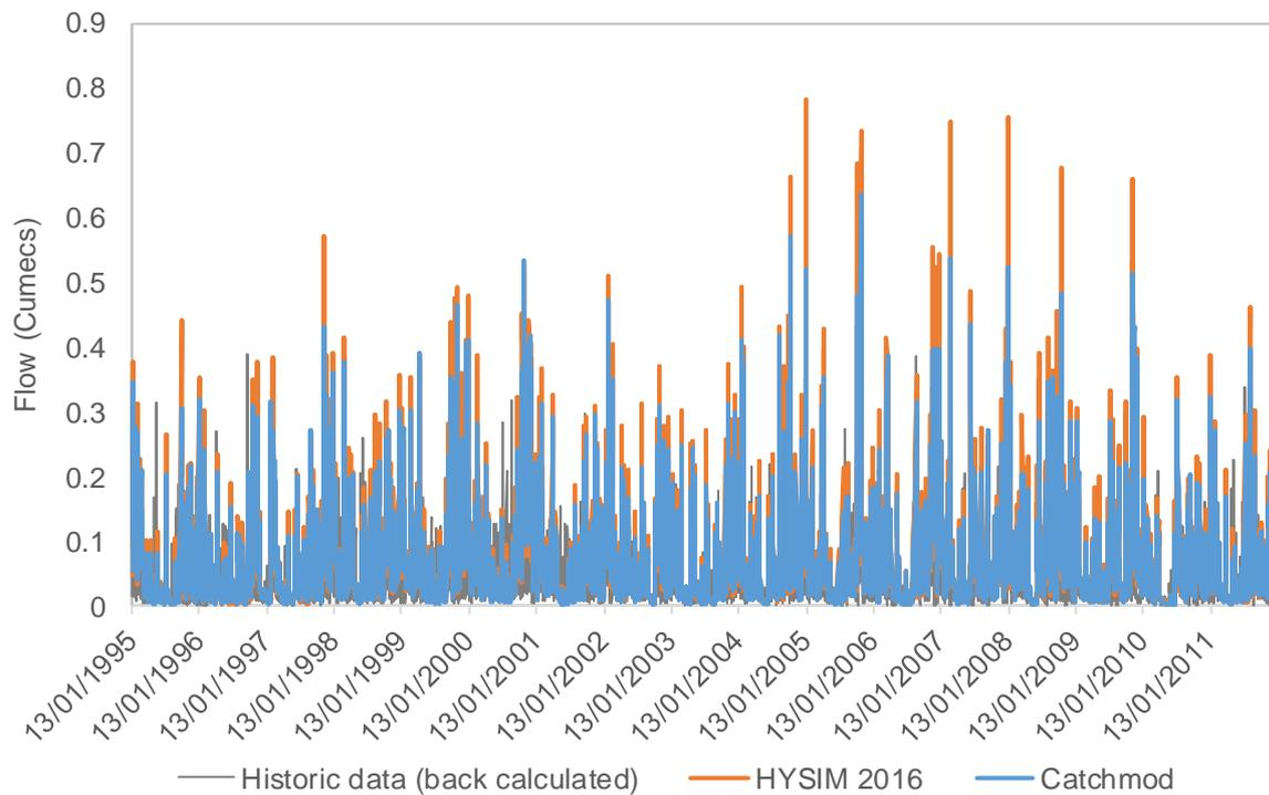
Figure 6.11 - Naturalised (back-calculated) and simulated (HYSIM 2016 and Catchmod) flows for Marchlyn Bach
