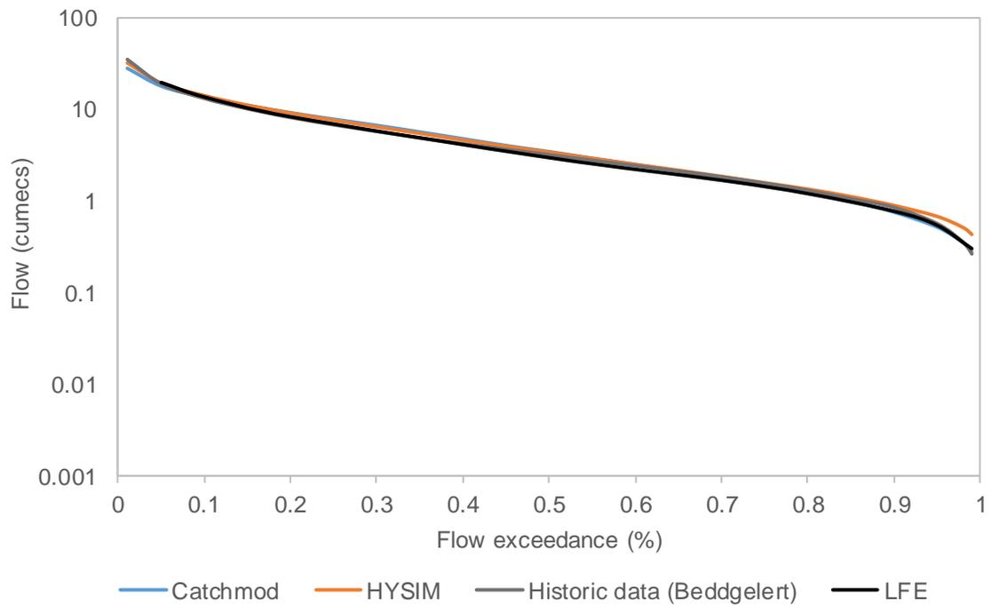
Figure 6.7 - Flow Duration Curves at Glaslyn for Catchmod, HYSIM, historic data (observed) and from LFE.
