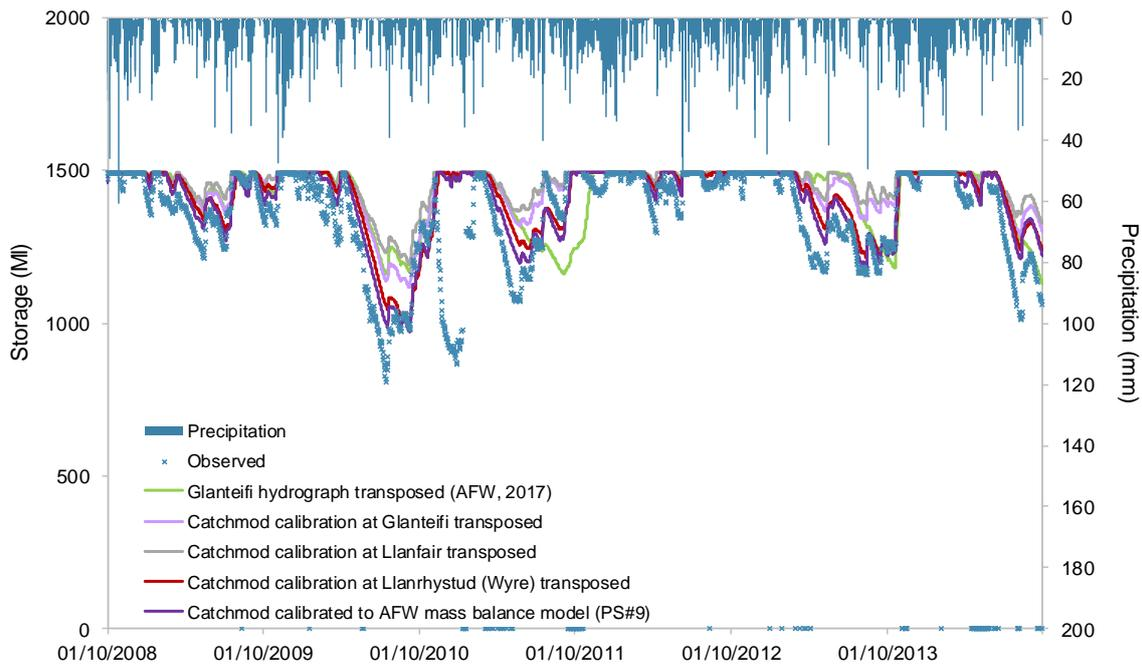
Figure B.11 - Observed and modelled storages for Teifi Pools for 10/2008 – 09/2014
