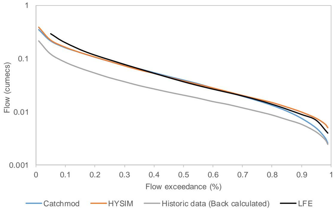
Figure 6.6 - Flow Duration Curves at Marchlyn Bach Llugwy for Catchmod, HYSIM, historic data (back-calculated) and from LFE.
