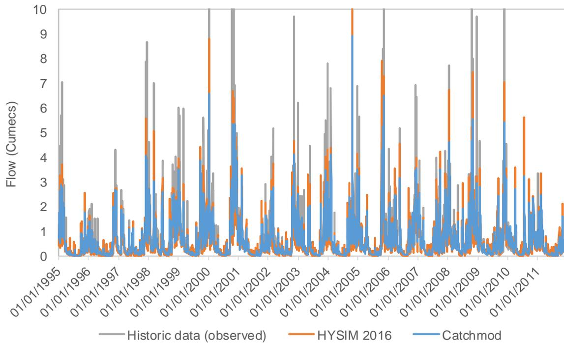
Figure 6.9 – Observed and simulated (HYSIM 2016 and Catchmod) flows for Llyn Cefni
