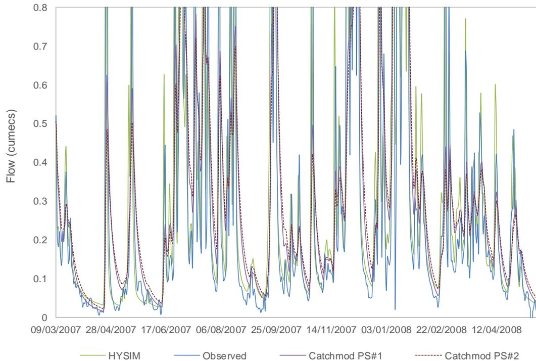
Figure 4.19 - Cwmystradllyn simulated and observed naturalised flows with focus on low flows
