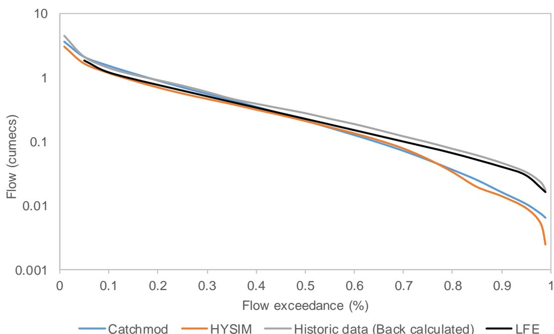
Figure 6.3 - Flow Duration Curves at Llyn Alaw for Catchmod, HYSIM 2016, historic data (back-calculated) and from LFE.
