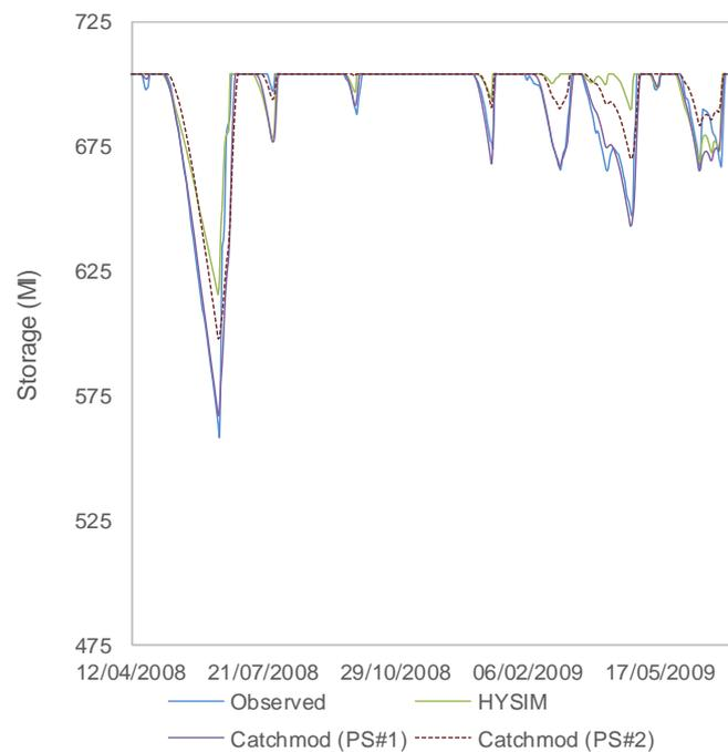
Figure 4.8 - Llyn Cwm Dulyn observed and modelled reservoir storages between April 2008 and June 2009
