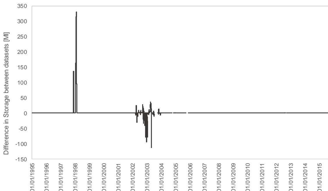
Figure 3.5 - Difference in storage between dataset sent by Gary Rowlands (Bodlyn Reservoir Levels with storage 1990-PRESENT DAY Amended.xlsx) and the AFW storage data.
