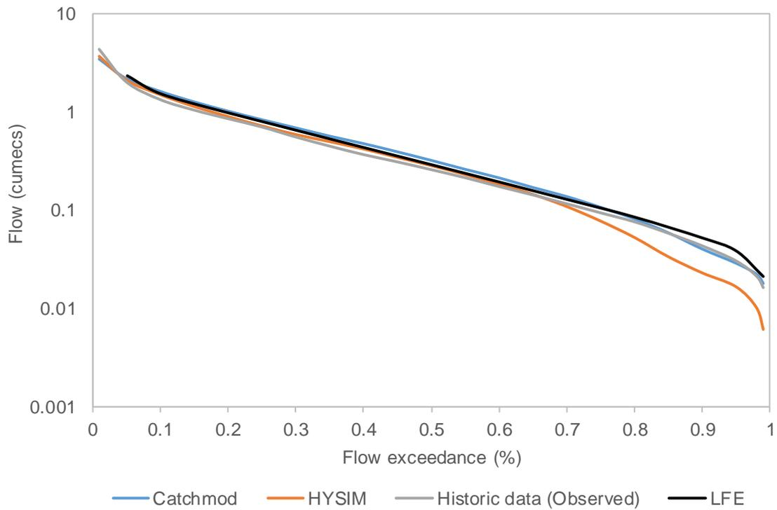
Figure 6.4 - Flow Duration Curves at Llyn Cefni for Catchmod, HYSIM, historic data (observed) and from LFE.
