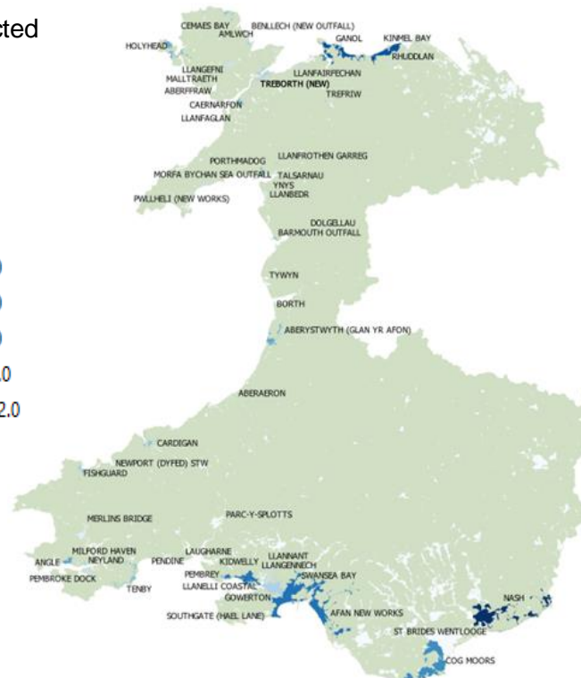
Figure 90 - Map of wastewater treatment work catchments impacted in the 1.25m sea level rise scenario.
